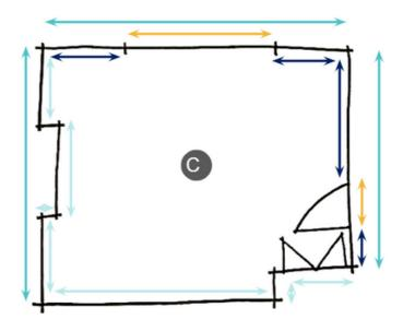
Note that all measurements should be taken from the interior face of the wall!
